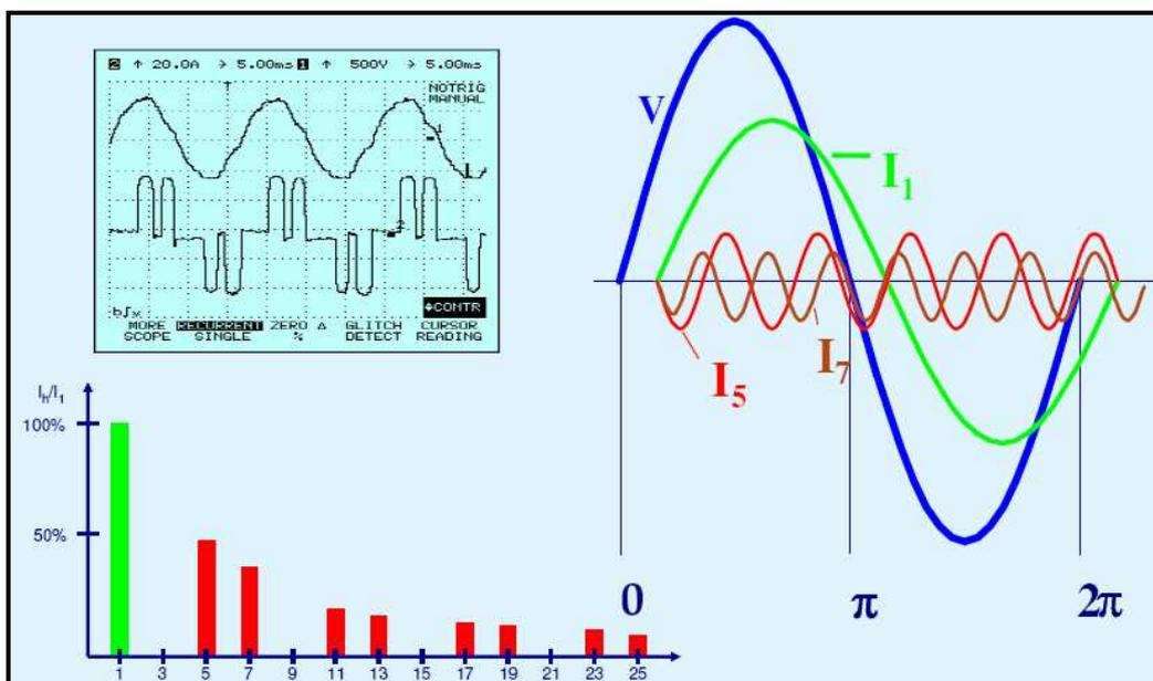
Figure 2. Harmonics existence lies to the phenomenon that current consists of components in frequencies multiple of the fundamental (50Hz)
